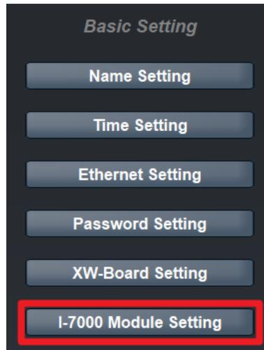
3. On the "I-7000 Module Setting Page", add I-7012FD module to the list (in this case, the I-7012FD locates at address 4). Click on the "Edit" button on the module list as indicated to edit the settings (for detailed module settings information, please refer to the user manual).
