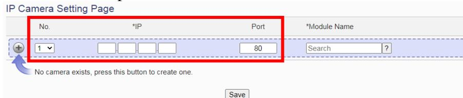
Figure 6-51 : Set up the No, IP address and Port of the IP Cameras
