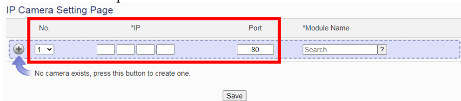
Figure 6-51 : Set up the No, IP address and Port of the IP Cameras
